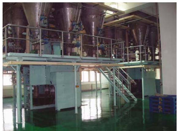
Dosing and weighing of an EME thin glass batch plant.
