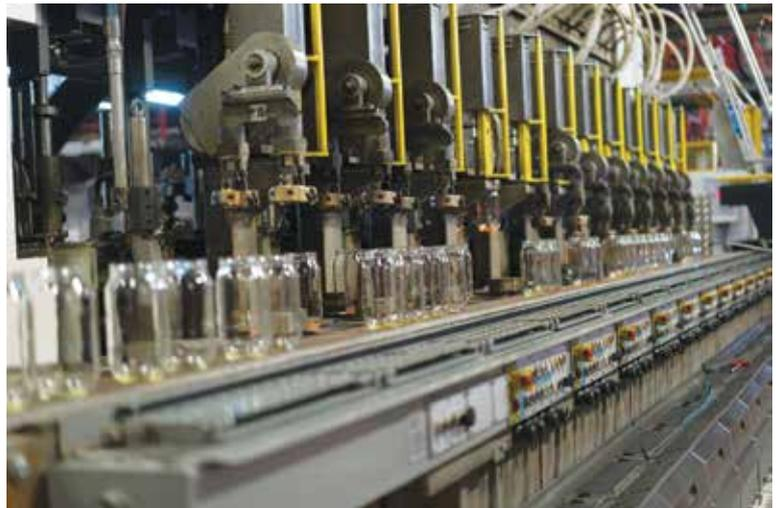
Two of the high speed IS machines have been designed for 6 1/4in double gob operation.
